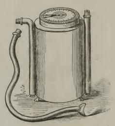
A spirometer, made upon the plan of the dry gas meter, has been for some time employed in Germany, and was introduced into use in this country by Dr. S. Weir Mitchell. It is altogether more simple in its management than the rather clumsy instrument of Hutchinson, and affords fully as accurate results. (Fig. 3.)
